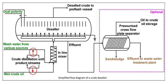
**Application:** On-Line monitoring of the salt content in crude oil by conductivity measurement.
