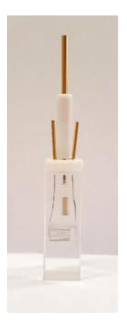
The cell includes also the platinum grid working electrode, the platinum counter and a silver/silver chloride reference electrode.
