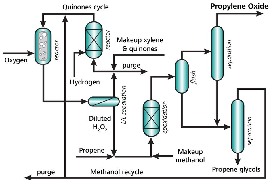
**Figure 11.** Schematic process diagram outlining the hydrogen peroxide-propylene oxide (HP-PO) method for byproduct-free production of PO. Adapted from Nijhuis et al.<sup>2</sup>
