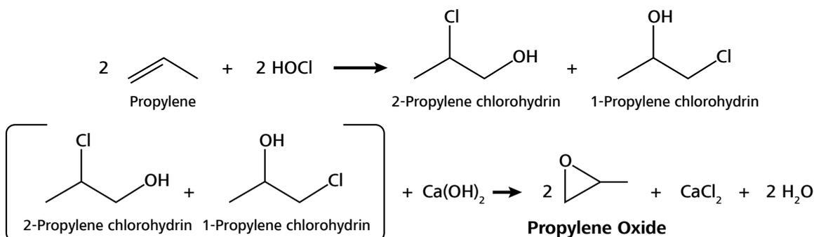
**Figure 1.** Chemical process behind the chlorohydrin route to produce propylene oxide. Adapted from Bernhard et al.<sup>3</sup>
