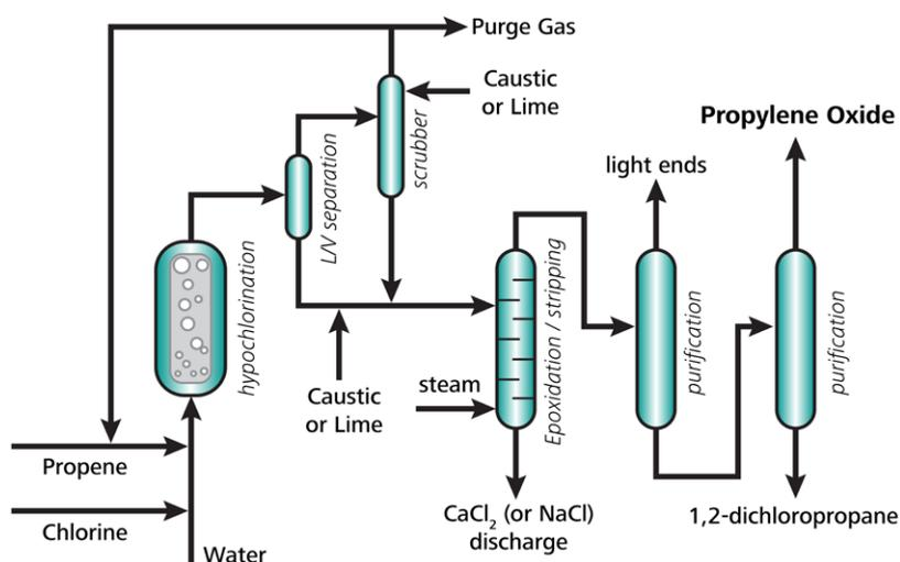
**Figure 2.** Schematic process diagram outlining the chlorohydrin method for co-production of propylene oxide. Adapted from Nijhuis et al.<sup>2</sup>
