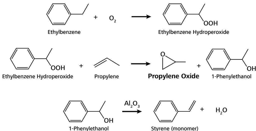
**Figure 3.** Chemical process behind the styrene (SM-PO) route to produce propylene oxide.<sup>3,4</sup>
