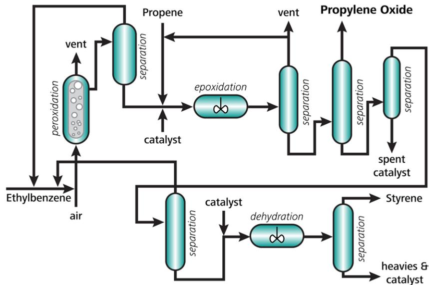
**Figure 4.** Schematic process diagram outlining the styrene method for co-production of propylene oxide. Adapted from Nijhuis et al.<sup>2</sup>
