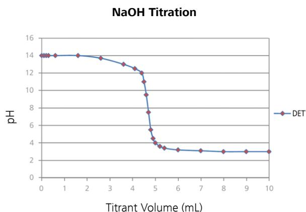
**Figure 12.** Titration curve for the determination of caustic soda (NaOH) in a chemical manufacturing process. Data provided by a wet chemical process analyzer from Metrohm Process Analytics.
