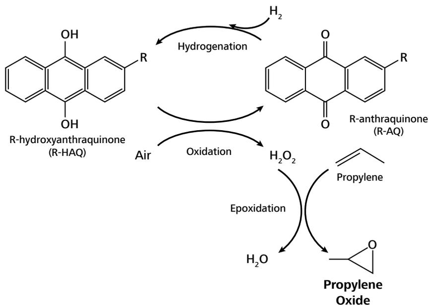
**Figure 10.** Chemical process behind the hydrogen peroxide route to produce propylene oxide.<sup>5</sup>
