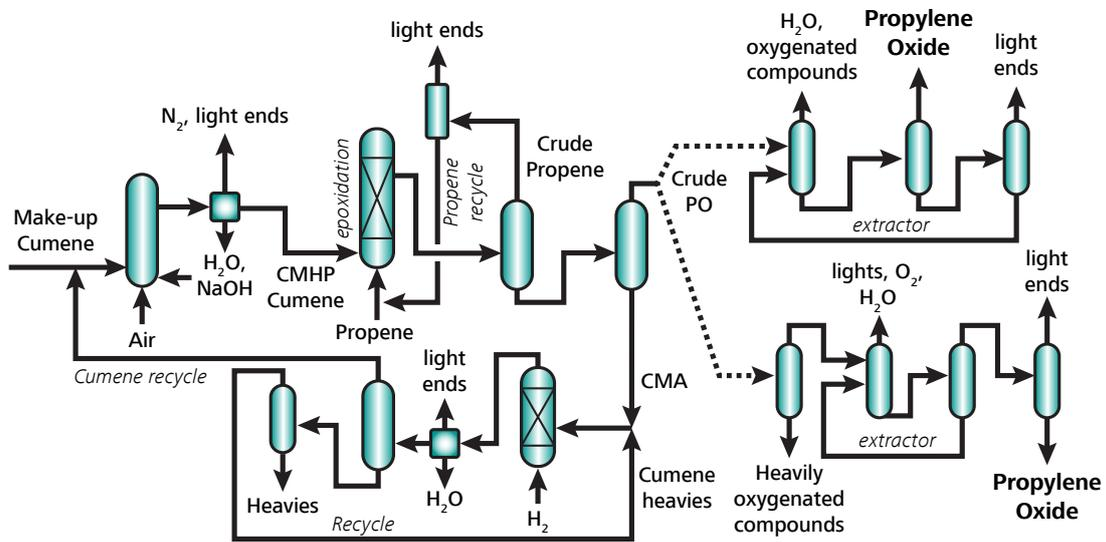
**Figure 8.** Schematic process diagram outlining the cumene-propylene oxide (CU-PO) method for byproduct-free production of PO. Adapted from Nemeth and Bare.<sup>7</sup>
