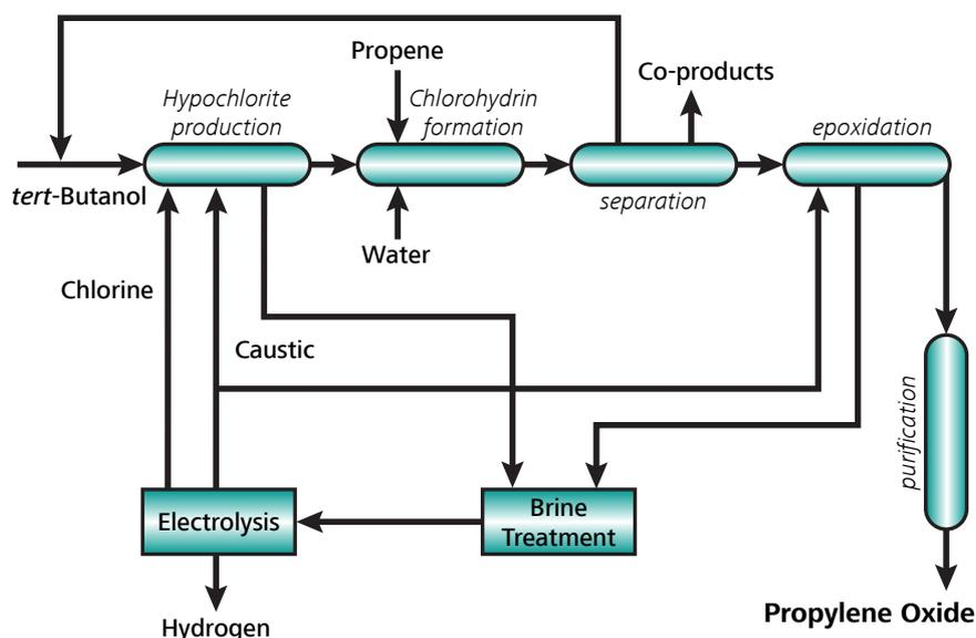
**Figure 6.** Schematic process diagram outlining the propylene oxide-*tert*-butyl alcohol (PO-TBA, also TBA-PO, MTBE-PO, or PO-MTBE in literature) co-production method. Adapted from Trent.<sup>1</sup>
