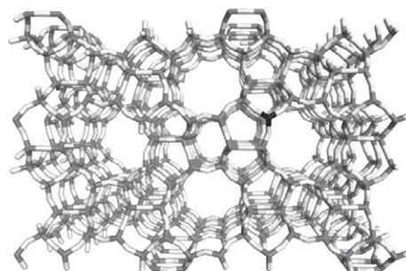
**Figure 9.** Structure of TS-1, Si (grey) and Ti (black) tetrahedral connected via oxygen bridges (white).<sup>8</sup>
