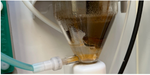
Figure 3. Not even biological growth inside the measuring cell disturbs the analysis. (Manual cleaning is suggested after 3 months.)
