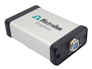
**µStat 200** is a small portable **Bipotentiostat** that can be applied for amperometric measurements at a fixed dc-potential as well as voltammetric measurements like differential pulse and square wave voltammetry. The supplied DropView software for Windows is used to control the instrument and to plot the measurements and perform the analysis of results. The instrument is controlled and powered by means of a USB connection.
