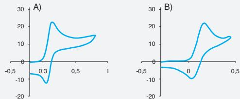
Ferrocene 2 mM in  $i\text{PrOH}$  and  $\text{LiClO}_4$  0.1M. A) Ref. C220AT, Screen-printed gold electrode / Ink AT (Aux.: Au; Ref.: Ag). B) Ref. C550, Screen-printed platinum electrode (Aux.: Pt; Ref.: Ag).
