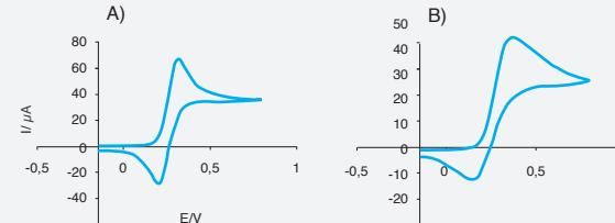
Ferrocene 2 mM in  $\text{CH}_3\text{CN}$  and  $\text{LiClO}_4$  0.1M. A) Ref. C220AT, Screen-printed gold electrode / Ink AT (Aux.: Au; Ref.: Ag). B) Ref. C550, Screen-printed platinum electrode (Aux.: Pt; Ref.: Ag).
