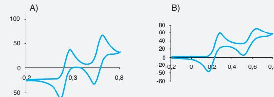
TTF (Tetrathiafulvalene) 2 mM in  $\text{CH}_3\text{CN}$  and  $\text{Bu}_4\text{NPF}_6$  0.1M. A) Ref. C220AT, Screen-printed gold electrode / Ink AT (Aux.: Au; Ref.: Ag). B) Ref. C550, Screen-printed platinum electrode (Aux.: Pt; Ref.: Ag).
