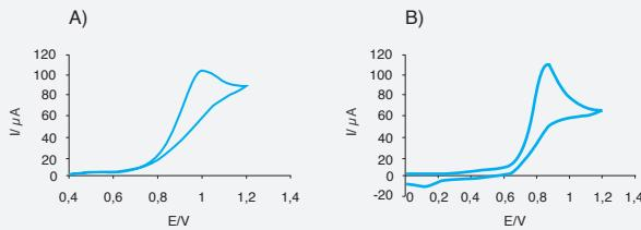
Hydroquinone 2 mM in  $\text{CH}_3\text{CN}$  and  $\text{Bu}_4\text{NPF}_6$  0.1M. A) Ref. C220AT, Screen-printed gold electrode / Ink AT (Aux.: Au; Ref.: Ag). B) Ref. C550, Screen-printed platinum electrode (Aux.: Pt; Ref.: Ag).
