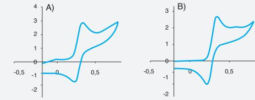
Ferrocene 0,2 mM in DMSO and  $\text{Bu}_4\text{NPF}_6$  0.1M. A) Ref. C220AT, Screen-printed gold electrode / Ink AT (Aux.: Au; Ref.: Ag). B) Ref. C550, Screen-printed platinum electrode (Aux.: Pt; Ref.: Ag).
