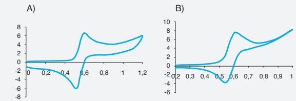
[2-phenylpyridinato-C2, N] iridium (III) 2 mM in  $\text{CH}_3\text{CN}$  and  $\text{Bu}_4\text{NPF}_6$  0.1M. A) Ref. C220AT, Screen-printed gold electrode / Ink AT (Aux.: Au; Ref.: Ag). B) Ref. C550, Screen-printed platinum electrode (Aux.: Pt; Ref.: Ag).
